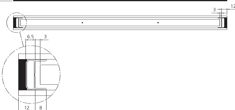
EXTRUDED "C" PROFILE SIDE GUIDE 22 x 6.5 mm
